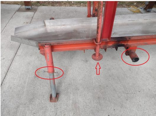
6. Remove conveyor belt from storage shed and mount top to dragon and bottom clamped to support on bench.
