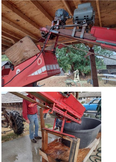
7. Attach motor coupling with hose and 2 alligator clamps.
