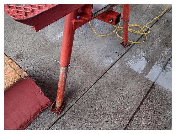
5. Raise the front and set the front jack supports. Insert the pin to hold the jack. Note the wheels are off and the hydraulically operated jack is retracted.
