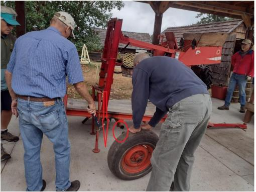
4. Raise the back end by hand and extend the rear jack supports, inserting the pins to hold up the jack.
